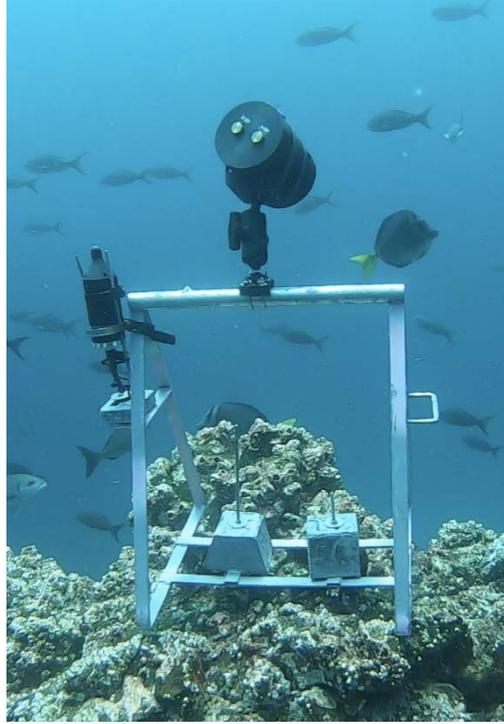
*Figure 3: Hydrophone (left) and long-term video camera (right) on stand*
