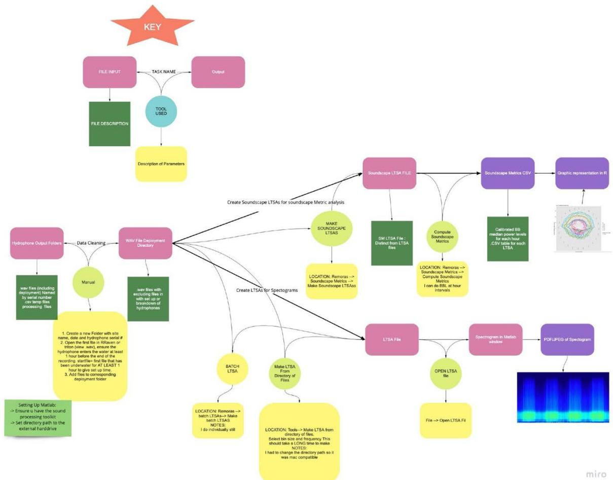
Figure 4: Workflow to convert deployment data into spectrograms and SPLs
