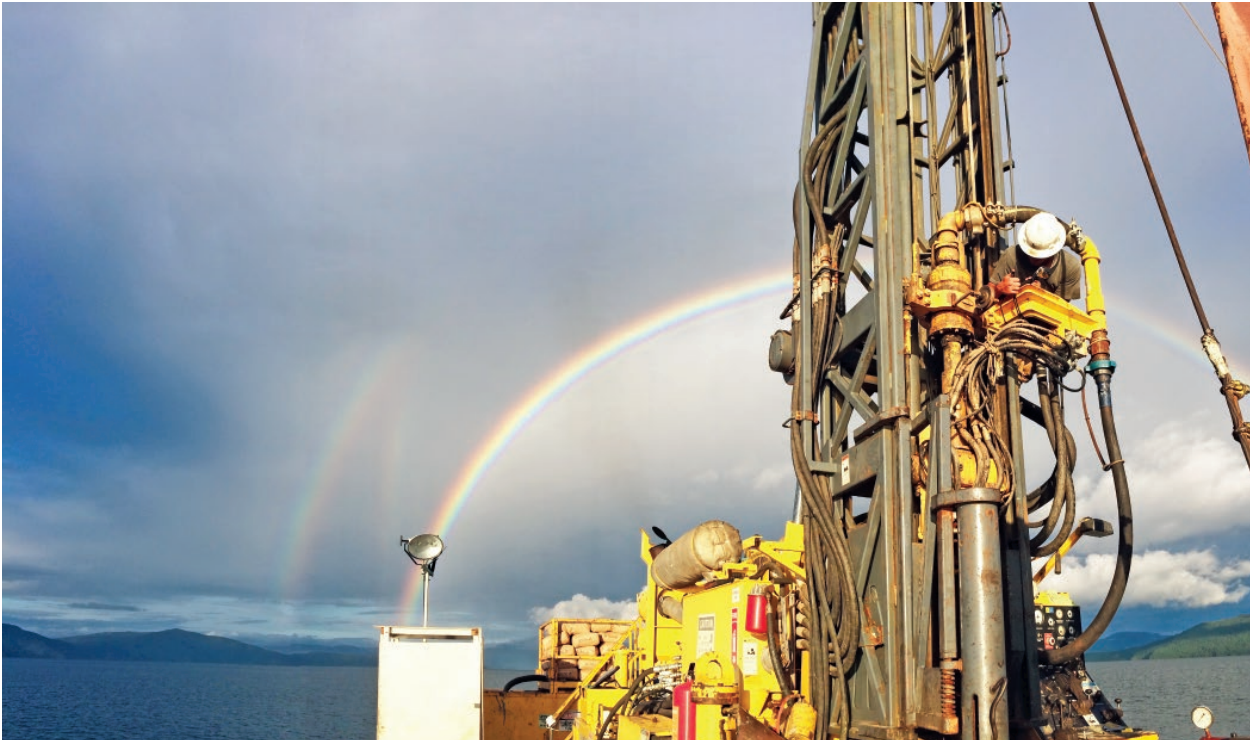
Jan Thorsten Blanke (Leibniz Institute of Applied Geophysics) prepares the drilling rig to log the geophysical properties of the borehole. This technique allows project scientists to recover physical and chemical information about the sediments in situ in the lake floor. Photo: Jim Russell
